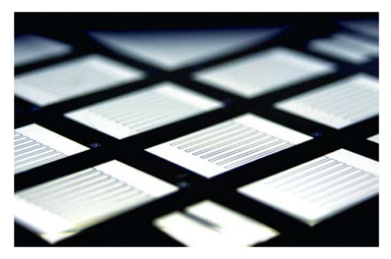
Back hetero: combshaped interlocking metal contacts on the back of rear-side solar cells with silicon heterocontacts. Several test cells on a silicon wafer can be seen.
