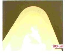
SCD tools represent the wave of the future and Synova's LMJ technology allows single crystalline diamond material to be machined with virtually no heat affected zone. Thus, a standard single point cutting tool retains its material qualities within its geometrical profile. The following three graphics show the edge waviness at the end cutting, nose and side cutting edges. At a magnification of 500, the edge waviness is less than 0.5 microns.
