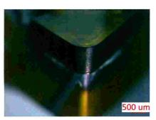
is best suited for the laser machining of SCD tool inserts. While cutting trenches are visible on the SCD insert, here brazed on to a holder, they have no impact on the surface roughness achieved on the workpiece.
