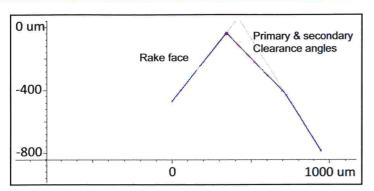
The Synova LCS 50-5 laser machining process delivers an extremely fine surface finish ( $Ra \le 1$  micron) for PCD tools, which eliminates the need for a second grinding operation.
